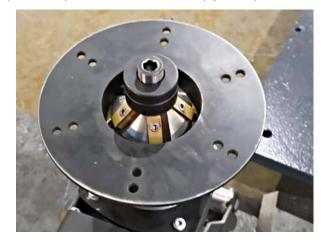
Unique blade size for tool holders with different angles
